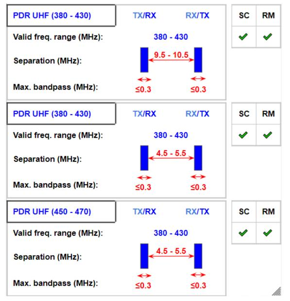
**Note:** For Simplex applications, the same Tx/Rx frequency can be used and the frequency pair spacing/separation rules do not apply.
