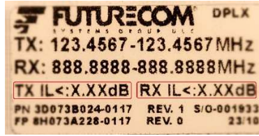
Figure 4: Duplexer Label (with indicated Insertion Losses)
