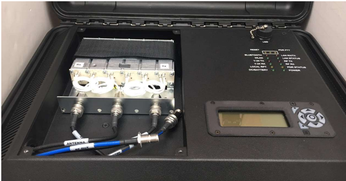
Figure 3: Internal Duplexer Cavity
