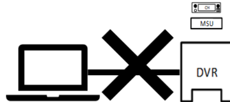
Figure 1 – No Physical Connection to VR
