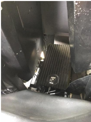
DVRS Installed Between Front and Rear Seat of Pumper Cab
