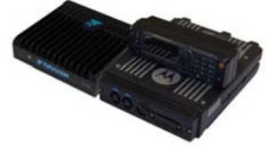
VRX1000 shown with Remote Mount APX™ 7500 with 07 Control Head (Mobile Radio Sold Separately)
